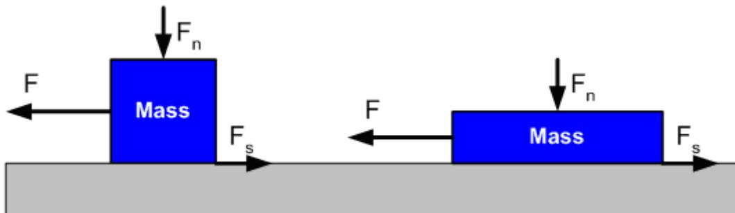
The blocks have equal mass and surface finish but one has twice the contact area of the other. If the blocks have a vertical force ( $F_n$ ) applied and are made to slide by the application of a horizontal force ( $F$ ) then a frictional force ( $F_s$ ) will resist the sliding.
