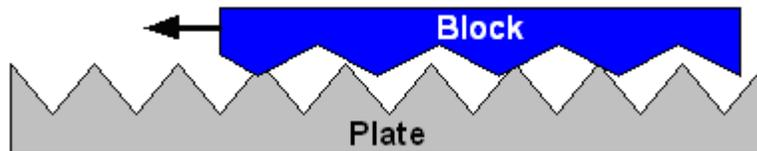
When movement occurs, the asperities rub against one another creating a natural resistance to movement as they slide over and deform one another. This resistance to the movement is the frictional force ( $F_s$ ) as defined by the equations above.
