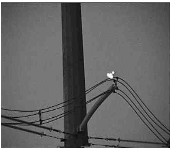
(a) Corona originating at the metal fittings of a 500 kV jumper line post NCI operating in a desert environment
