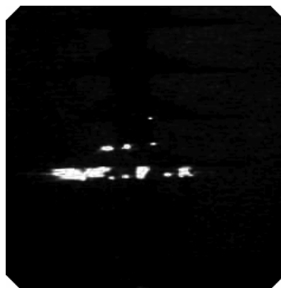
(c) Corona from water drops on weathershed at 50 kV (0.75 p.u)
