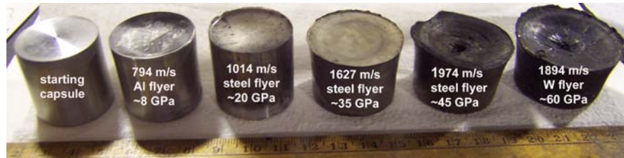
Figure 3: Deformed capsules recovered after experiments. The BMG sample material is inside the capsules.
