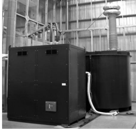
Figure 3. UQAC 350 kV alternating high-voltage system
